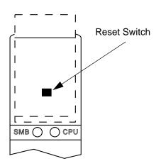
Figure 2-5. The Reset Switch
